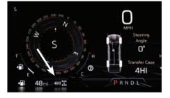
▶ If a shift cannot be completed, the transfer case returns to the last chosen setting. The current 4-wheel-drive status is displayed on the Driver Information Center.
