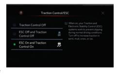
**Note:** StabiliTrak will turn on automatically if the vehicle exceeds 35 mph unless Off-Road, Terrain or Baja mode is enabled and active.
