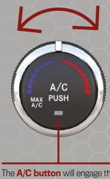
The **A/C button** will engage the Air Conditioning (A/C) system.
