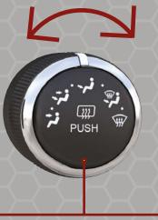
The **Rear Defrost button** will turn on the rear window defroster and heated outside mirrors (if equipped).
